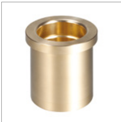
MFB 2102.71 Soilde Bronze Material: CuZn25Al5Mn3Fe3 Housing tolerance recommended H6
