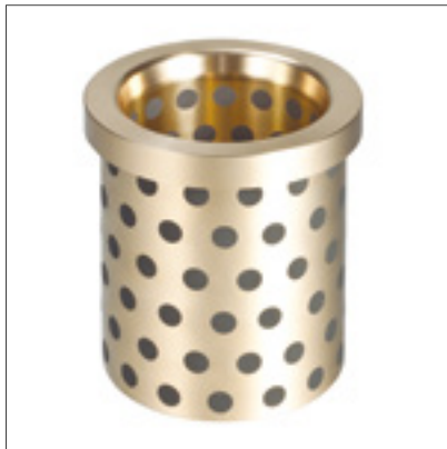
MFB 2102.70 Material: CuZn25Al5Mn3Fe3 +Graphite (500#SP) Housing tolerance recommended H6
